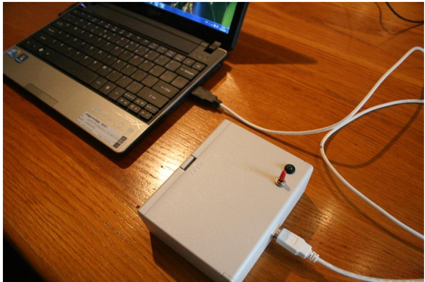
Ninthway NTM programming station for wireless programming of NTMs in application connected to a PC via USB.
